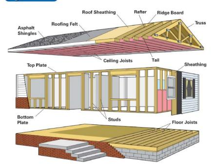
Whole House This drawing shows the major structural elements of a house. Why might a house with framed rafters have more useful attic storage than a house with roof trusses?
